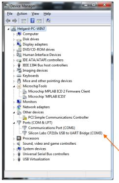
5. USB interface with a Personal Computer (PC) A CP2102-GM USB to UART Bridge interfaces between a PC and the UART on the MCU. It may be necessary to install an appropriate driver on the PC if it is not handled automatically by the operating system. The driver can be found here:
