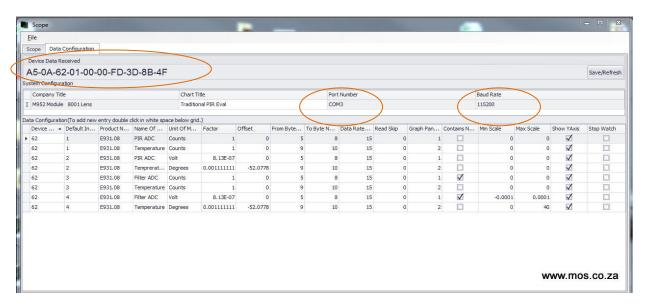
Ensure that the correct Port and baud rate is also set for the module.
