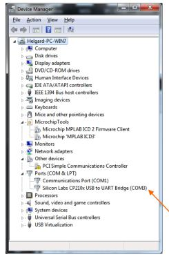
5. USB interface with a Personal Computer (PC) A CP2102-GM USB to UART Bridge interfaces between a PC and the UART on the MCU.
