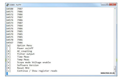
The 'f' was pressed to show the filtered ADC values. Software filters are implemented on the module for all devices except the E931.08.
