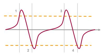
The threshold for motion sensing is usually set between 100 and 200 uV
