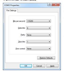
The software on the module is able to interface to a terminal with the following settings for the port.
