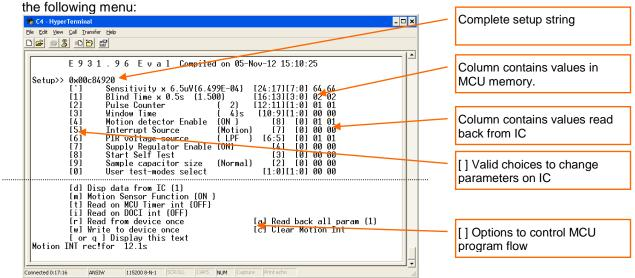
Note that all of the registers that are described in the datasheet are on the upper half of the terminal display, on the bottom half is controls for program flow.
