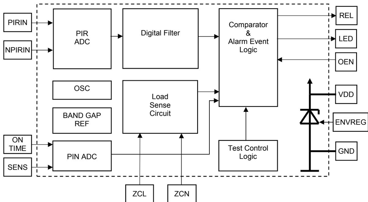
Fig 1: Block diagram of M931.98
