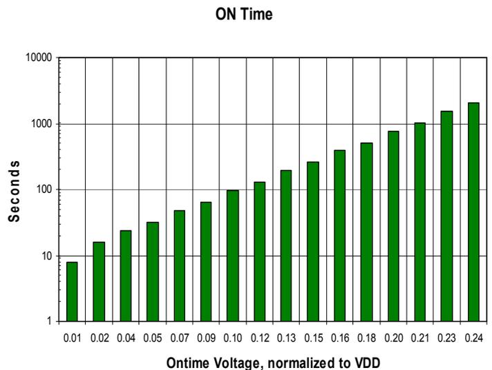
Graph 2: REL Output On Time in seconds vs. ONTIME pin voltages normalized to VDD.
