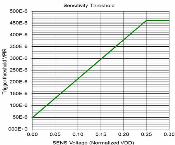
Graph 1: PIR voltage trigger threshold vs. SENS pin voltages normalized to VDD.
